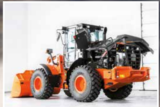
Easy access for maintenance from ground level.
