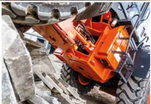
The optional belly guard provides added protection.
