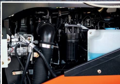
Fuel efficient Cummins engine, with NO DPF.
