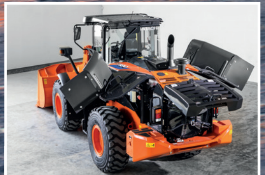
Ground level access for easy maintenance.
