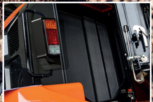
Standard anti-clogging radiators (WPFR)
