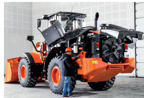
Easy access to the engine compartment.
