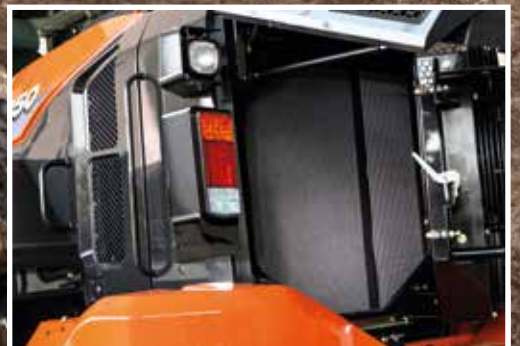
Optional anti-clogging radiators enhance durability.
