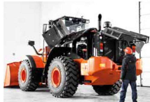
Easy access to the engine compartment.
