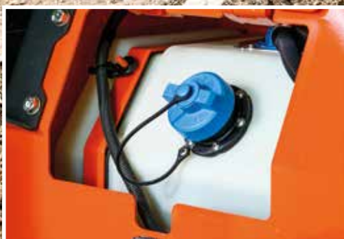
The urea tank is located for safe and easy access form ground level.
