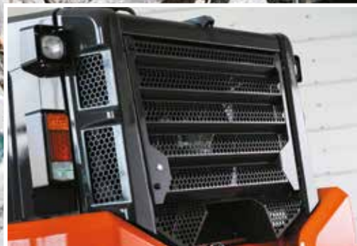
New rear grill protects radiator compartment.
